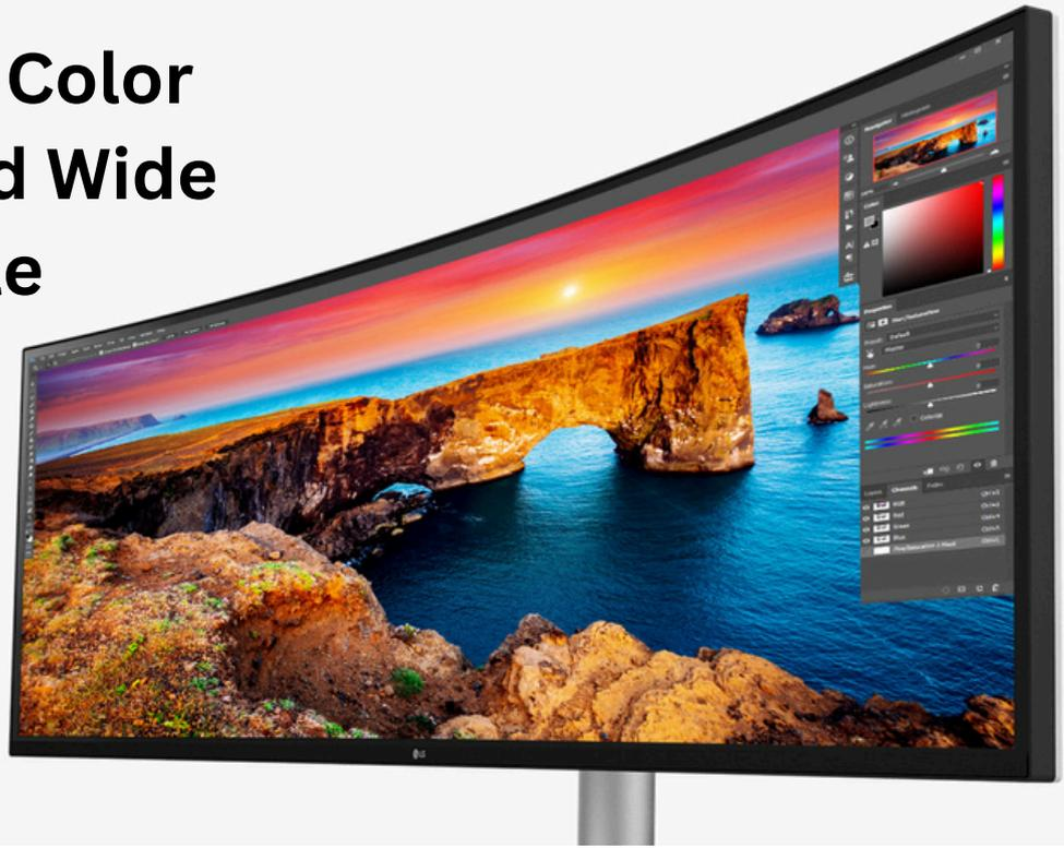
It is an UltraWide 32:9 Dual QHD (5120x1440) monitor with a doubled 27-inch 16:9 QHD pixel space in one screen. With 70% more pixels compared to 32:9 FHD resolution (3840x1080), you can go beyond multitasking with a multi-format multiplex.
